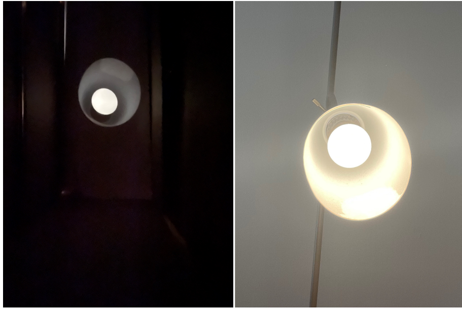
Figure 4: (Left) Image of the scene captured with the pinhole camera with a very small aperture. (Right) Image of the same scene when captured with a smartphone camera.
